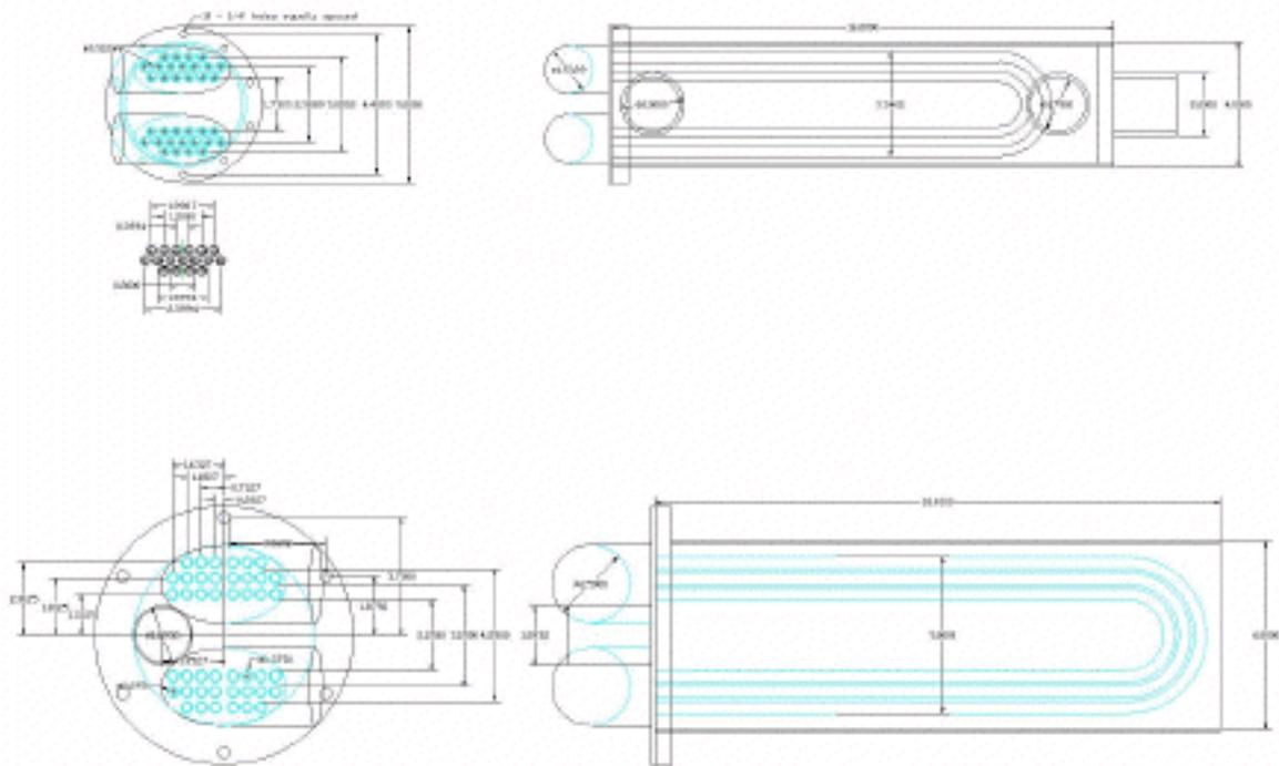
Figure 2. Detail drawing of exhaust/intake heat exchanger.
