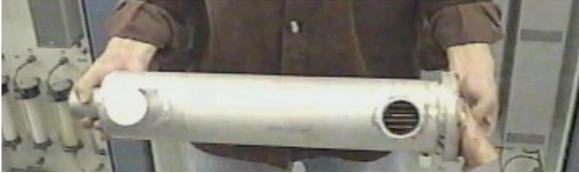
Figure 4. Photograph of assembled exhaust/intake heat exchanger.
