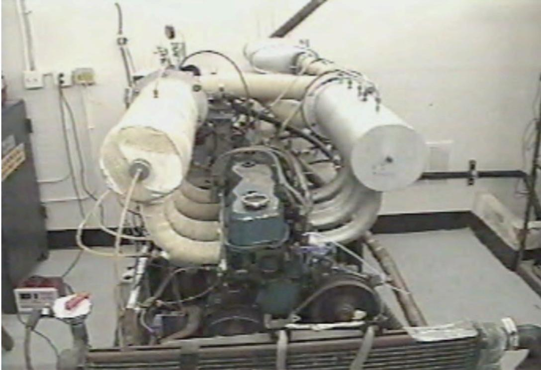
Figure 6. Photograph of engine with installed intake / exhaust heat exchanger (front view).
