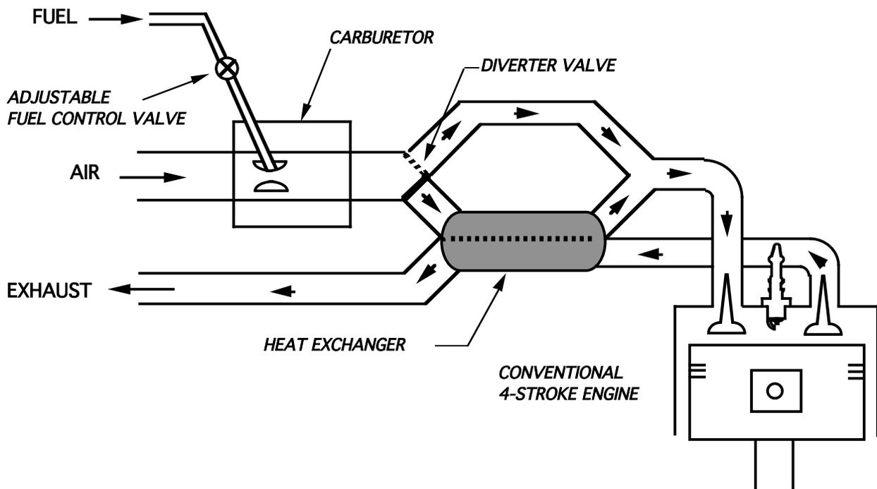
Figure 17. Possible implementation of TPCE using heat exchanger and diverter valve to control inlet temperature and thus torque output. (Carbureted gaseous fuel system shown; liquid fuel system would likely employ fuel injection system).
