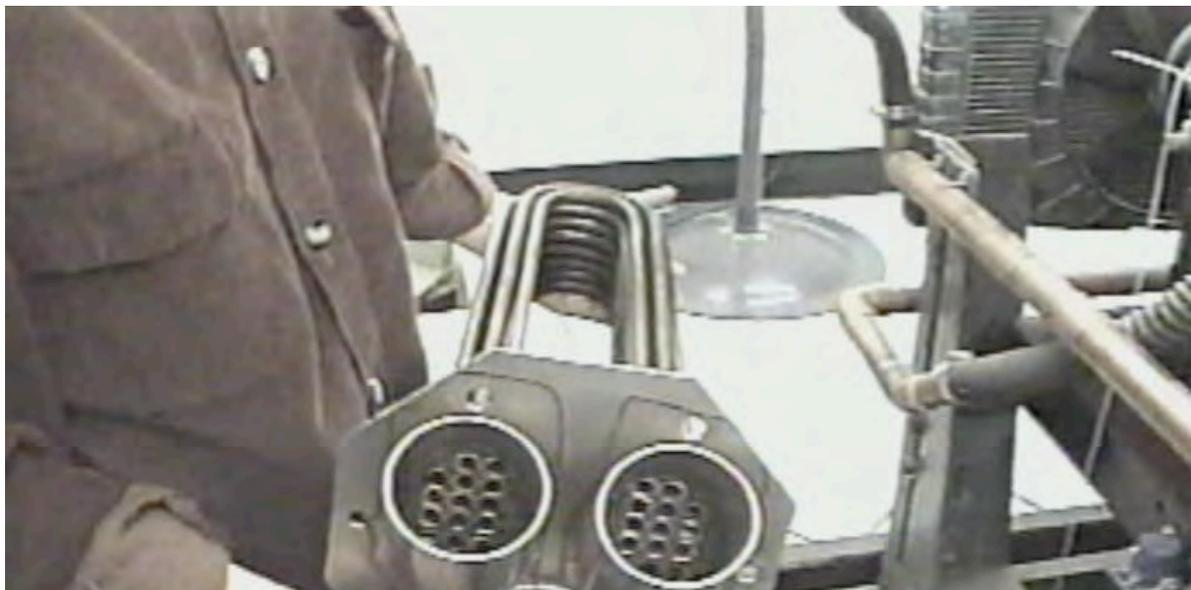
Figure 3. Photograph of interior of heat exchanger. Intake air flows through U-shaped tubes.
