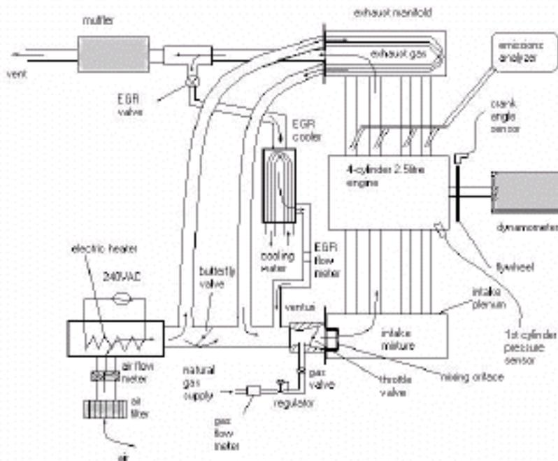
Figure 1. Schematic diagram of engine test setup including exhaust/intake heat exchanger.
