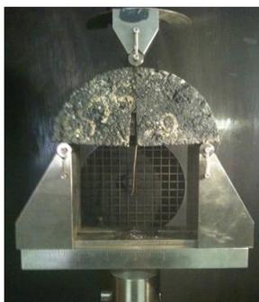
Figure 1, SCB test, Cross head Movement Method
