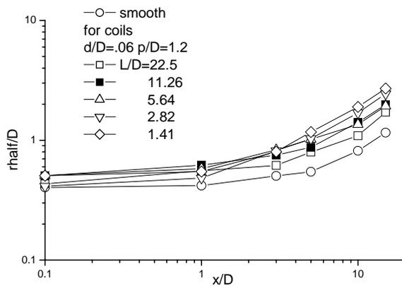
Figure 6. Axial decays of the flow center mean velocity and axial turbulence intensity and axial variation of the jet half widths. Uncertainty in  $r_{half}$  is  $\pm 0.05$ , in  $\frac{U_m}{U_0}$  is  $\pm 0.005$ , and in  $u'_c/U_0$  is  $\pm 0.02$  at 20:1 odd.
