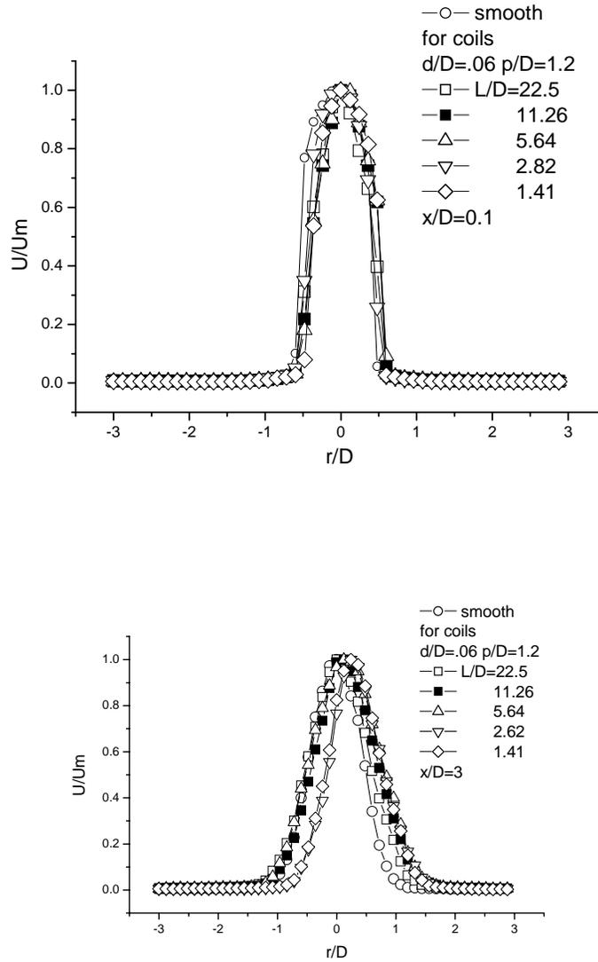
Figure 4. Radial variations of normalized axial mean velocity at  $X/D = 0.1$  and 3. Uncertainty in  $\frac{U}{U_0}$  is  $\pm 0.005$ , in  $\frac{r}{D}$  is  $\pm 0.05$ , and in  $X/D$  is  $\pm 0.05$  at 20:1 odd.
