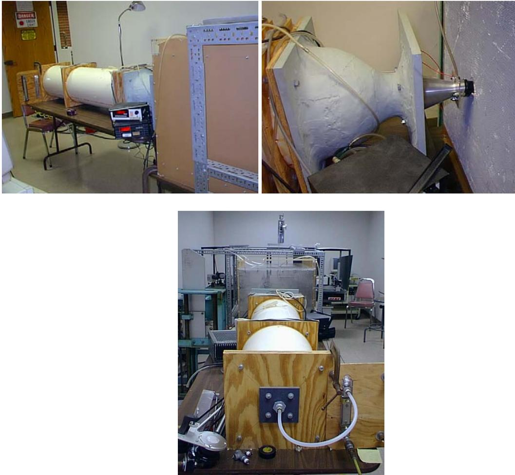
Figure 1. The open jet facility.
