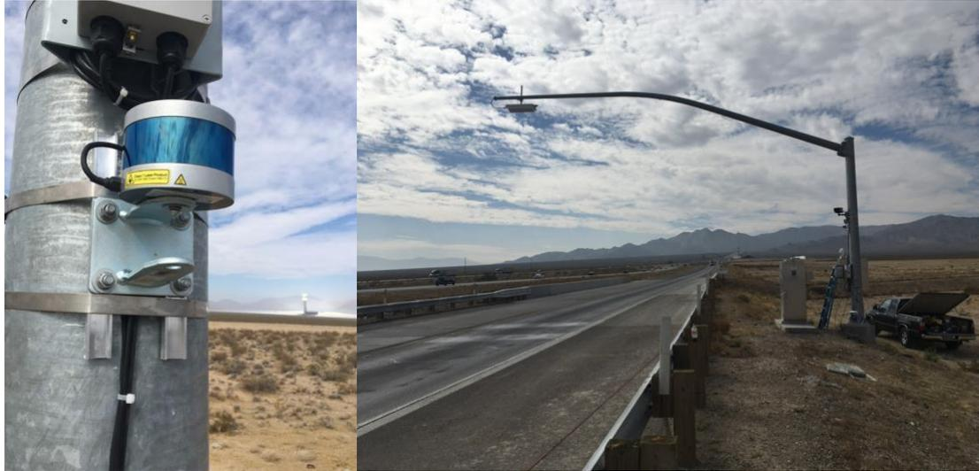
*Figure 2. LiDAR installation on I-15 for a PSR project under PI Stephen Ritchie (UCI).*
