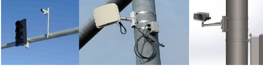
Figure 2. Examples of modern traffic sensing technologies: from left to right — video detection system, radar, and solid-state LiDAR.
