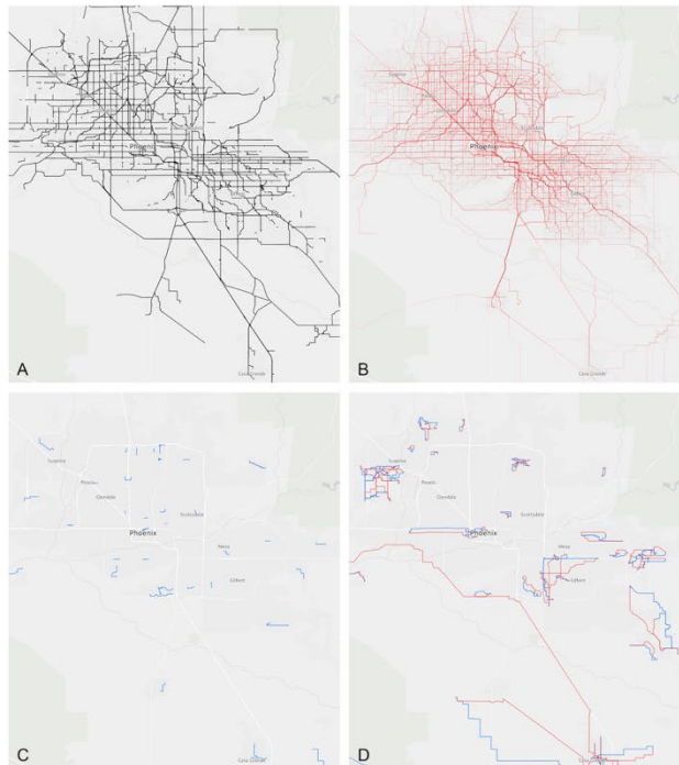
Figure 2. Outcomes of 10% centrality-based disruption simulations in Des Moines, Philadelphia, Las Vegas, and Phoenix showing: a) disrupted nodes, b) disconnected trips, c) unaffected trips, d) rerouted trips. Red lines are shortest paths before disruption and blue lines are shortest paths after disruption
