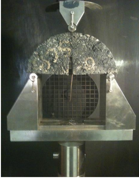
Figure 3 Set-up of semi-circular bend test
