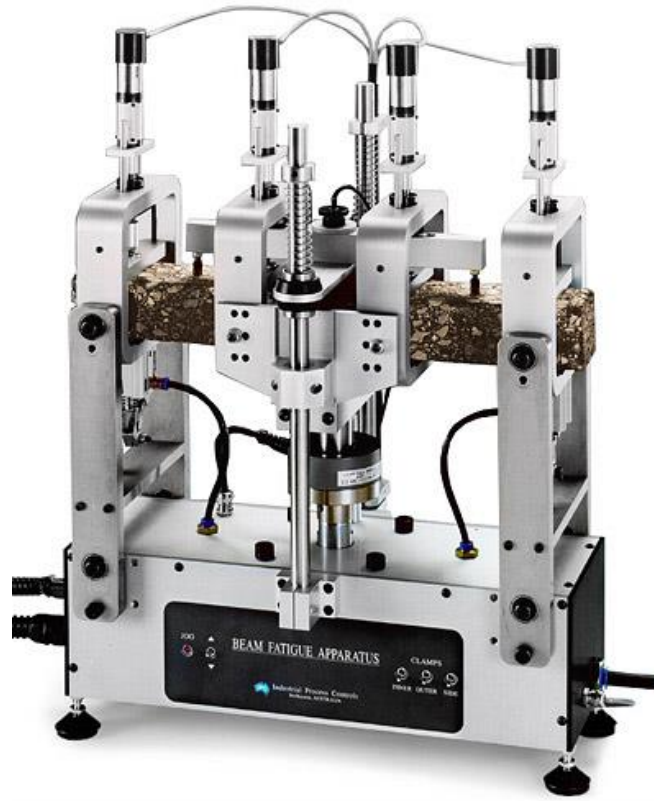
Figure 4. Fatigue Beam Test (Courtesy of Inopave Inc.)
