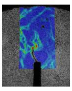
Figure 2, SCB test, Non-Contact Camera method
