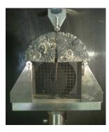
Figure1, SCB test, Cross head Movement Method
