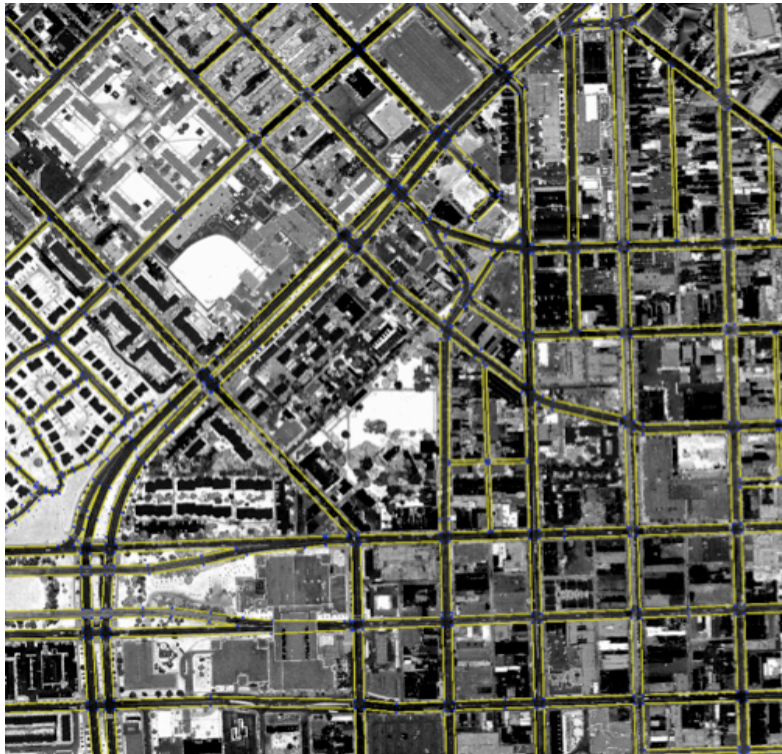
Figure 24: (a) Extracted roads of portion of Baltimore downtown from LiDAR, and (b) road attributes (widths, centerlines, and intersections).
